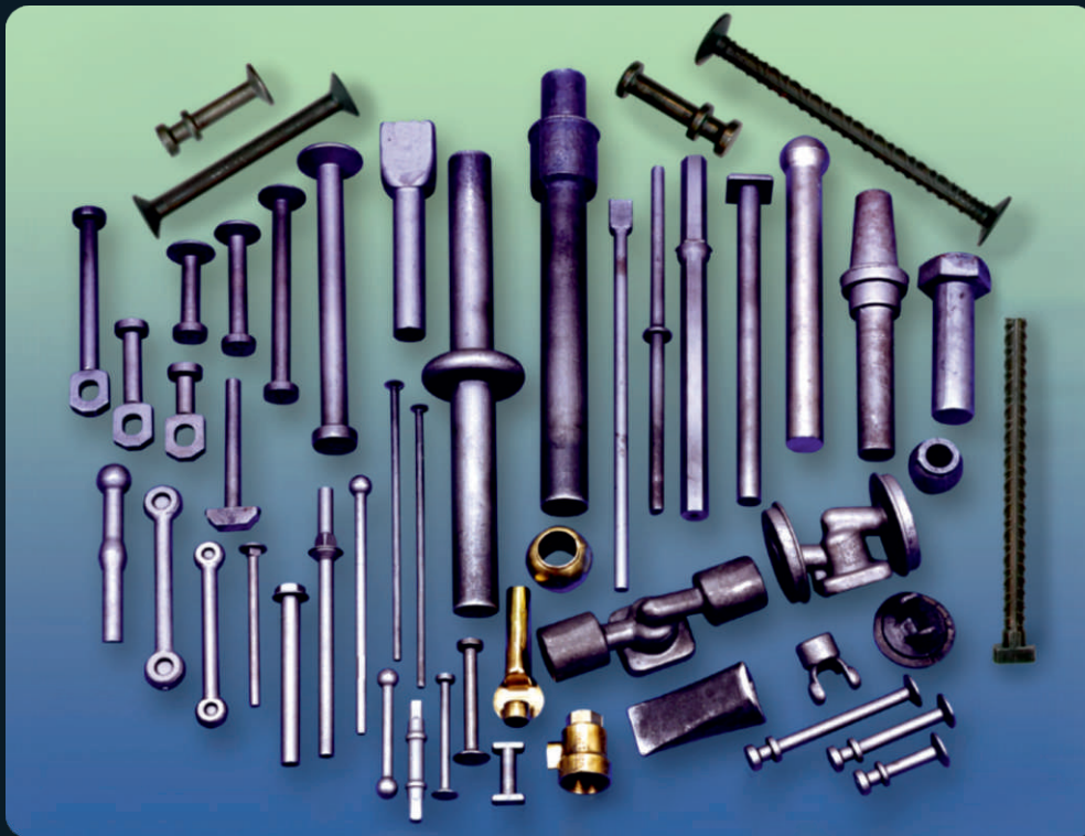
Forgings made in special forging devices
